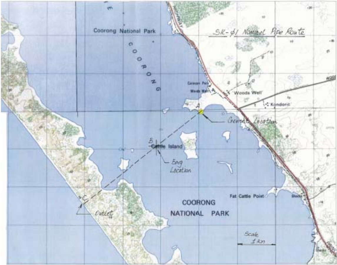
Figure 6. Proposed location of pumping infrastructure (source: Tonkin Consulting 2009)].
